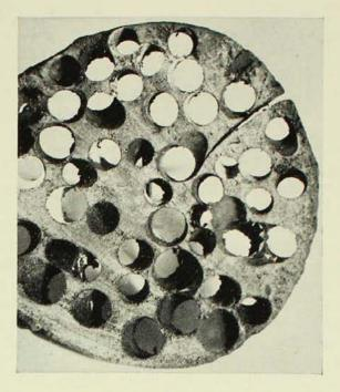
Left: A juvenile Cobra borer (greatly enlarged) exposed in its burrow in a chip of softwood (Oregon fir). One of the pair of shells at the head or boring end of its body is clearly seen. The processes at the tail end act as plugs to seal the minute holes in timber surfaces made by the borers when they first enter as larvae. Above: A thin cross-section of piling, showing the effect of a heavy attack by Cobra borers on non-resistant timber.
